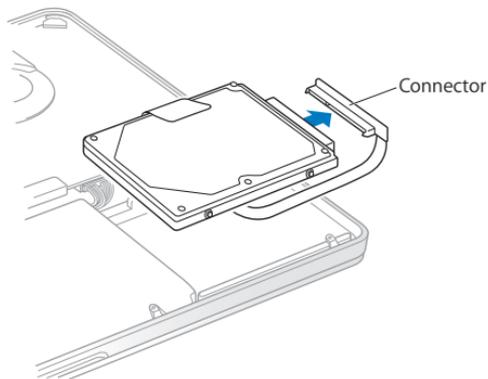
The connector is attached to a cable and remains in the hard disk drive bay.
