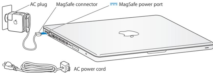
To extend the reach of your power adapter, replace the AC plug with the AC power cord. First pull the AC plug up to remove it from the adapter, and then attach the included AC power cord to the adapter, making sure it is seated firmly.
