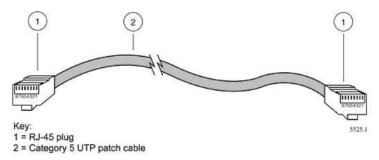
Figure B-6: Category 5 UTP Cable with Male RJ-45 Plug at Each End
