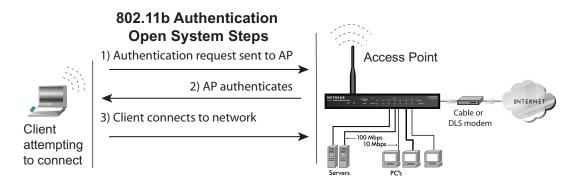
Figure 7-1: Open system authentication
