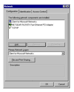
You must have an Ethernet adapter, the TCP/IP protocol, and Client for Microsoft Networks.
