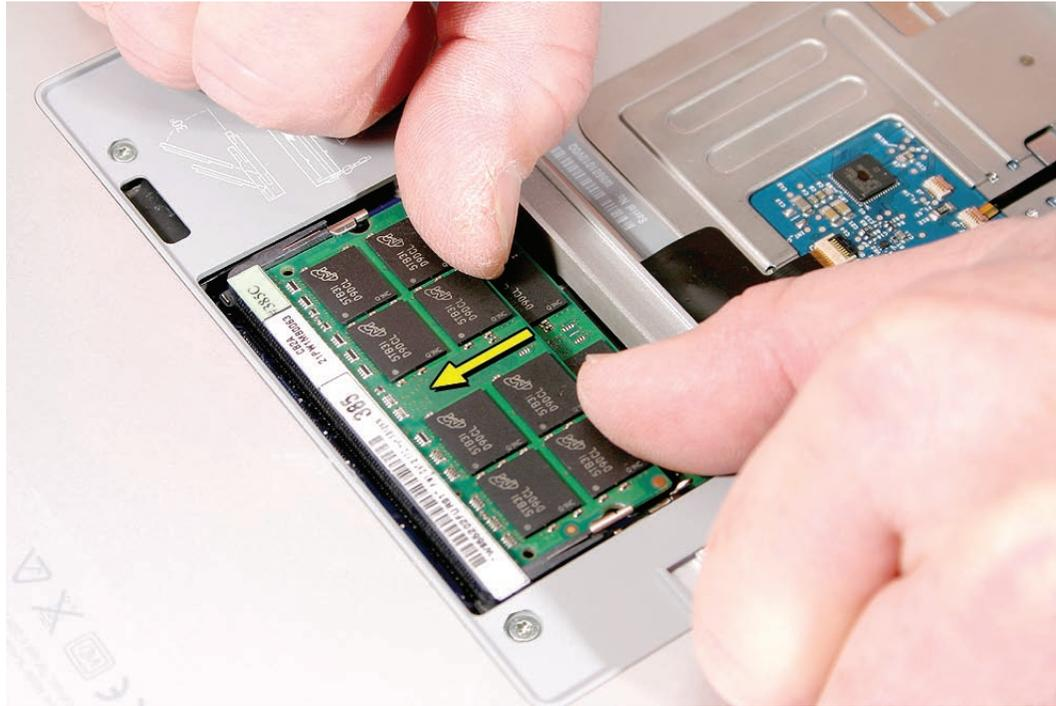
6. Check that the cards are secured by the brackets on both sides.
