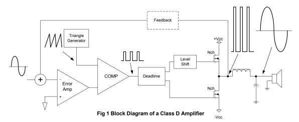
Fig 1 above shows the basic block diagram for a Half Bridge Class D amplifier, with the waveforms at each stage. This circuit uses feedback from the output of the half-bridge to help compensate for variations in the bus voltages.
