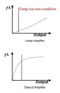
Fig 3 Linear and Class D Amplifier Efficiencies
