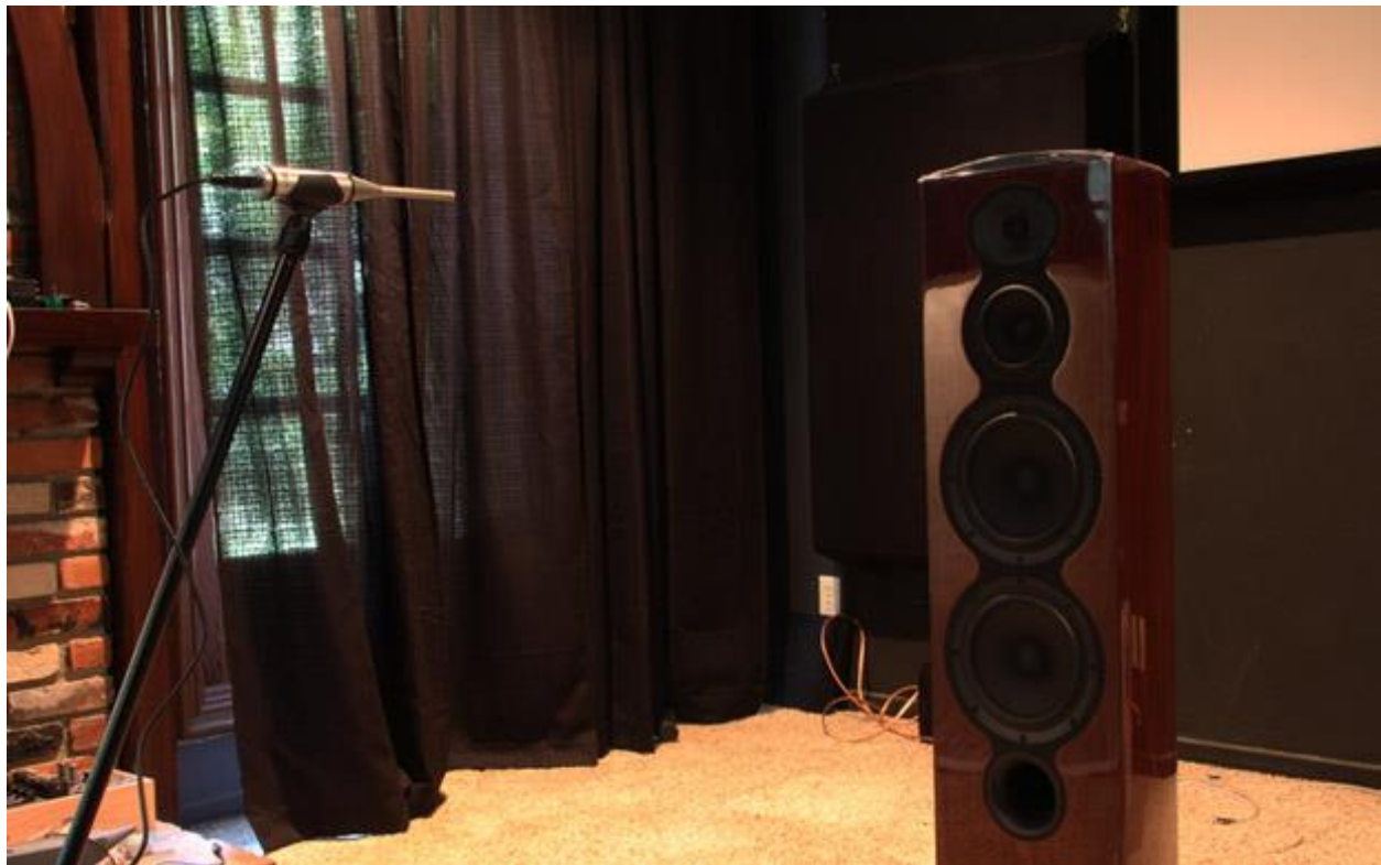
Measuring the Revel F208 at a distance of 1 meter in the author's listening room. Don't do this.
