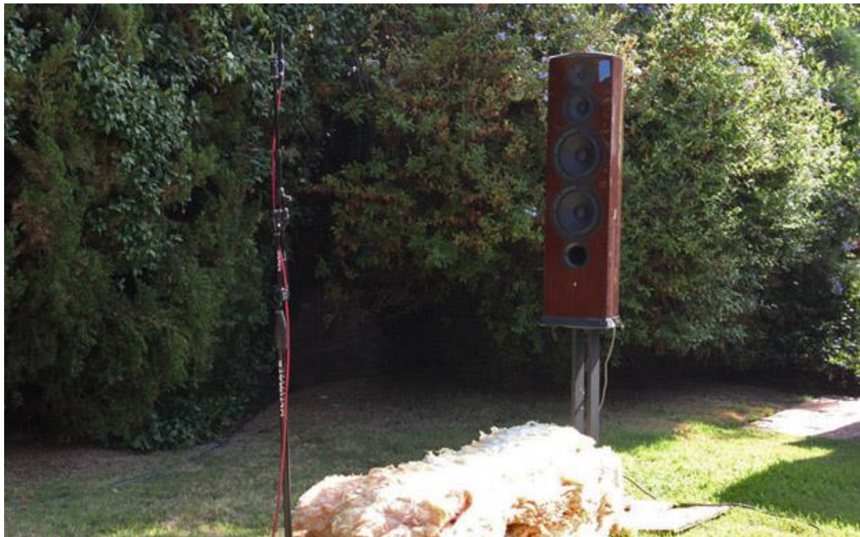
Measuring the F208 in the author's backyard using quasi-anechoic technique
