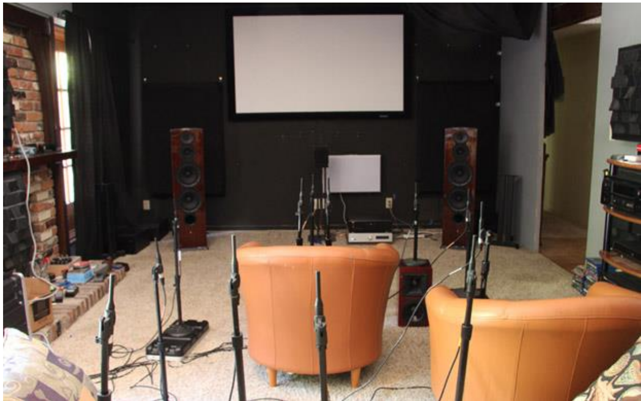
Measuring the F208 in the author's listening room using averaged in-room technique
